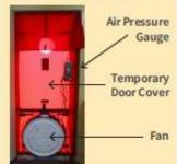
We perform a blower door test to identify how much air leakage is in your home by depressurizing it with a special fan mounted to a temporary door. A smoke tracer and infrared camera then help to locate leaks.
